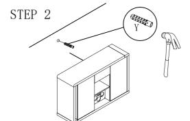
1. Use a light harmer to tap anchor into hole. 2. Anchor should fit snugly. If hole is too small, drill again to increase hole size . Do not force anchor into wall.
