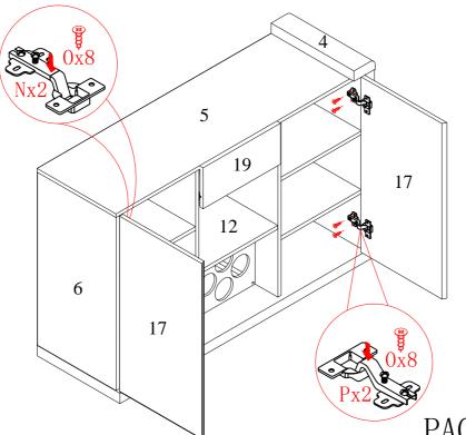
To adjust the door in or out,loosen this screw and push the door further in or push further out then retighten screws.
