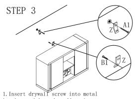
bracket and into drywall anchor.
